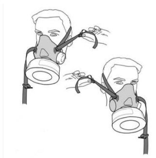
TIGHTEN EACH STRAP ALTERNATELY TO CLAMP THE MASK
